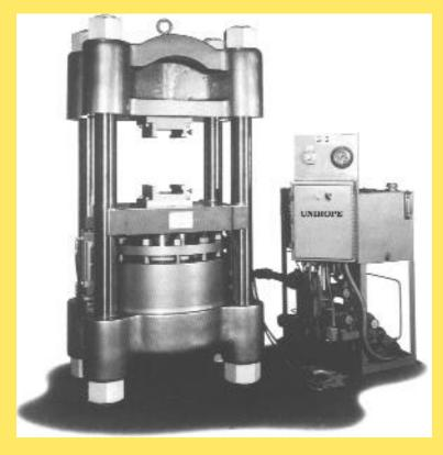
1500 ton swager for wire rope flemish eye slings up to 2-1/2" diameter. One of a total of 8 rope swagers to meet any and every demand.
