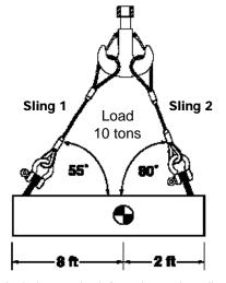
From the calculation on the left we know that sling 1) is tensioned to 2 tons, and sling 2) is tensioned to 8 tons. However both slings are on an angle, hence we must apply the angularity factor for EACH sling:
