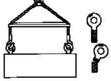
Never reeve slings through eye bolts. This alters the load and the angle of loading.
