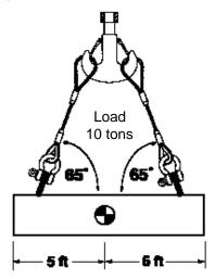
In this example the 10 ton load is equally centered between the pick points but we lift at a sling angle of 65°. We know that each sling is subjected to 5 tons VERTICALLY. In applying the calculation from the previous section (Angularity)we arrive at
