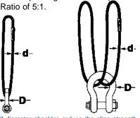
Small diameter shackles reduce the sling strength and, most likely, that small diameter shackle also has insufficient capacity for that job. Shackle or not, objects to be lifted and all hook up points MUST at least ensure a D/d Ratio of 5:1.
