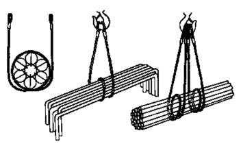
The same principle as above, but here we use a plain double wrap hitch. Both sling eyes are placed into the load hook. You do not have to consider choker hitch reduction factors, but when loads get wider you may have to reduce the sling capacity due to the angularity factor.
