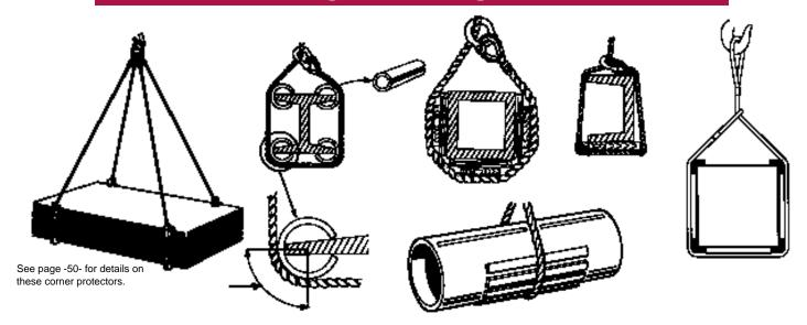
**U**se proper corner protection. A sharp steel edge will cut through any wire rope sling; at least it will permanently damage the sling. Sliced steel pipes have proven to an effective corner protector. For square and round objects proper wooden padding will be sufficient. Before making the final lift do a trial lift and check if the padding is strong enough and does not crack under the load weight.
