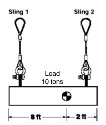
When the center of gravity is not equally spaced between the pick points, the sling and fittings will not carry an equal share of the load. The sling connected to the pick point closest to the CG will carry the greatest share of the load.
