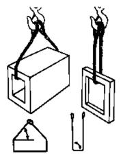
When using a basket hitch you must take the sling angle into account. Make sure the load is properly padded to prevent sling damage.
