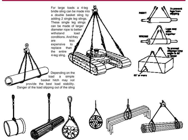
Standard choker hitches provide better load control as long as the loads are short. When lifting longer bundled loads there is the danger that some of the bundle content may slide out of the sling. As can be seen, a standard choker hitch compresses the load from three sides only A better way to do the same lift. Use a double wrap choker hitch and for long loads use 2 slings. The double wrap compresses the load on all 4 sides and provides far better load control.
