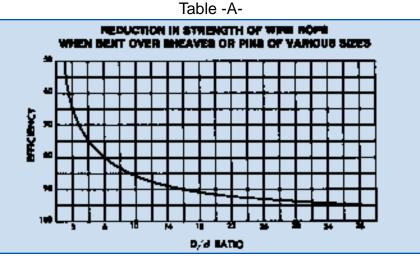
When a wire rope is bent around any sheave or other object there is a loss of strength due to this bending action. As the D/d ratio becomes smaller this loss of strength becomes greater and the rope becomes less efficient. This curve relates the efficiency of a rope diameter to different D/d ratios. This curve is based on static loads and applies to 6-strand class 6x19 and 6x37 wire rope.
