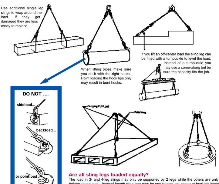
balancing the load. Unequal length sling legs may be one reason, off-center or buckling loads another. <u>YOU</u>, the user, must evaluate each lift taking into consideration the type of load, and the type of sling. Same capacity sling legs will stretch unequally if loaded unequally. All wire rope sling capacity tables (e.g. in ASTM B30.9 and Wire Rope Users Manual) consider ALL legs sharing EQUAL loads.
