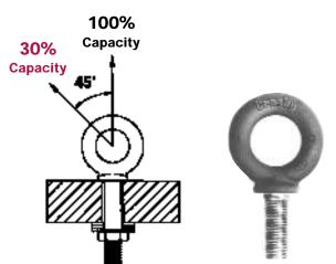
AT 45° lifting angle eye bolts have just 30% of their rated VERTICAL capacity. A sling (any type) used at the same 45° angle retains 71% of it's vertical capacity.
