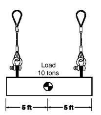
When lifted vertically the load will be shared equally if the center of gravity is placed between the pick points. If the weight of the load is 10 tons, then each sling will be subjected to a tension of 5 tons. Required is a 3/4" diameter, 6-strand IWRC wire rope sling.
