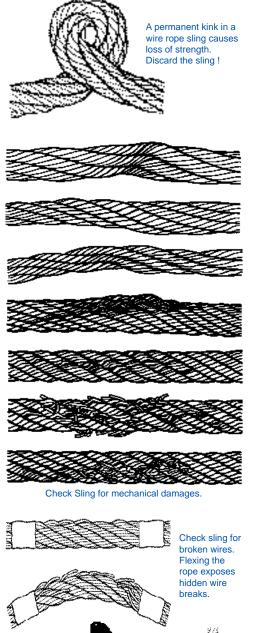
Inspect the bearing point of the eye. Check for deformation and wear of sleeve, thimbles, and all attached hardware. Check for broken wires where the rope enters the sleeve or socket.
