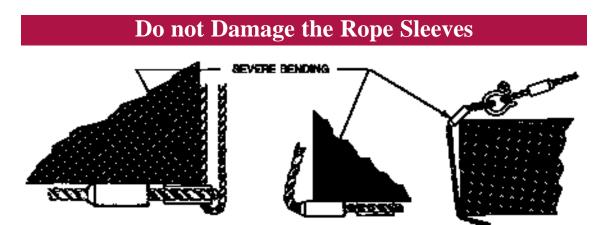
**D**o not place the splice sleeves, rope thimbles, or sling hooks around corners. A sleeve failure under these condition will result in the failure of the sling and you WILL drop the load. Check the sleeves regularly for nicks and cracks. Rope sleeves are NOT designed to be hooked under loads and be used as a swaged button; rope sleeves secure the rope ends and are not intended to lift the load. DO NOT WELD ANYTHING ONTO THE ROPE SLEEVE OR TO ANY ROPE END ATTACHMENT.
